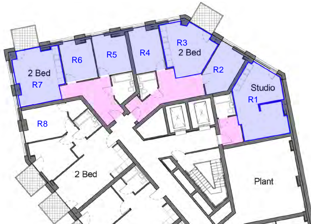
Figure 1 Annotated extract from first floor plan of North Island Building No. 3 (drawing no. TH-IS_ZZ_001_A_16092_(P00)_P101 rev. P00). Room references in blue font (R1, R2, etc.) are those used by Point 2 in its impact assessment. Rooms shaded blue are habitable rooms that take light from over the Site. Areas shaded pink are hallways/circulation spaces.
